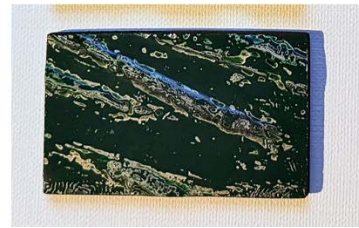
Fig. F8. Layering structure of lacquer surface without cloth mounting
