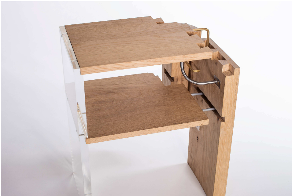
Figure 3. Commode model used for testing mount options and exploded elements. Photography by Dominic Mifsud ©Victoria and Albert Museum, London
